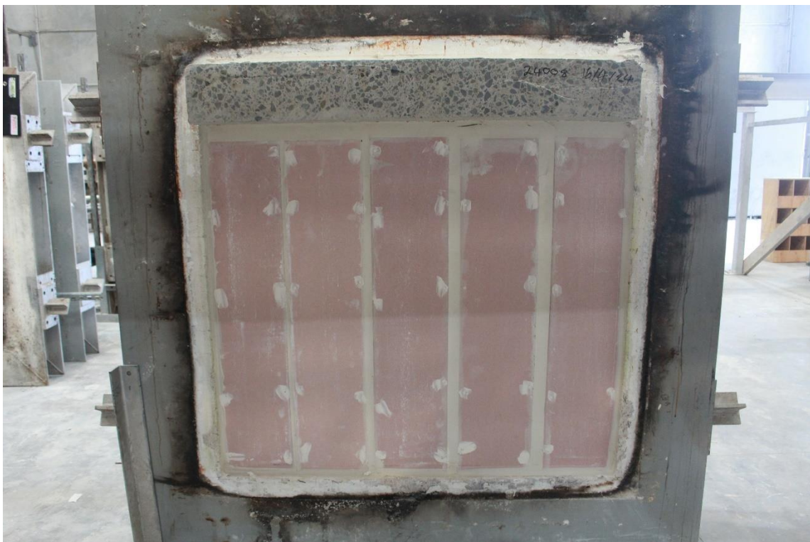
Figure 12 – Exposed face prior to test commencement
